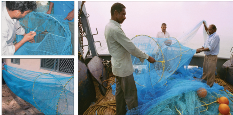
Figure 6 Views of JFE-SSD under fabrication (upper left), ready for installation (lower left) and its operation (right).
