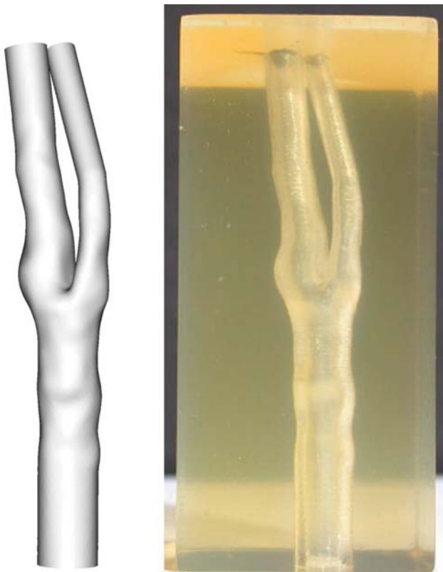
Fig. 6 Left patient-specific model of a carotid bifurcation used as input for the RP system (see Appendix). Right picture of the physical phantom
