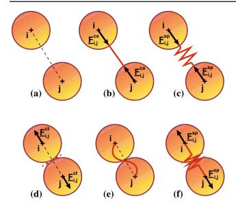
Fig. 1 Schematic drawing of the three interactions between particles: a-d contact inducing compression force when the particles touch, b-e cable inducing tension force when longer than its initial length and c-f spring inducing compression or tension force when, respectively, shorter or longer than its initial length
