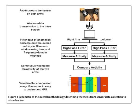
MATLAB is used for *online* analysis and data visualization. The sensitivity of the on board ST accelerometer is  $\pm 2g$ .
