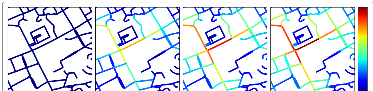
Figure 4 The evolution of the system towards equilibrium when the static risk is taken to be proportional to betweenness. The parameter values are \eta = 0.4 , \Gamma = 0.5 and \omega = 0.7 , and the value of \delta t used in the simulations is 0.01.
