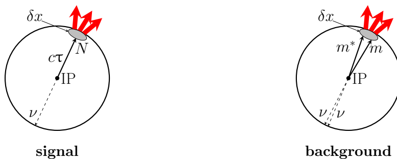
Figure 5. Schematic illustration of the signal , that is given by the decays of a heavy neutrino at a distance c\tau from the interaction point. The SM background is given by two light neutrinos ( \nu\nu ) and two long-lived mesons m and m^* , which decay sufficiently close to each other, such that only one secondary vertex can be resolved. The detector resolution \delta x is dependent on the detector component.
