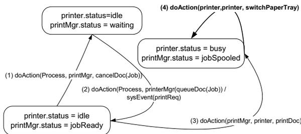
Figure 4: State chart for Printer system functionality.
