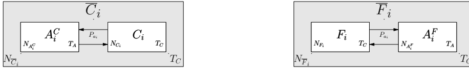
Fig. 4 Left: coherence state \bar{C}_i expanded to show sub-states A_i^C and C_i . Right: forward state \bar{F}_i expanded to show sub-states A_i^F and F_i . The average number of robots in each state is shown as N ; T_A is the number of time steps spent in the avoidance states A_i^C and A_i^F .
