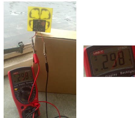
Fig. 20. Rectenna measurement in a typical indoor ambience with a voltage meter
