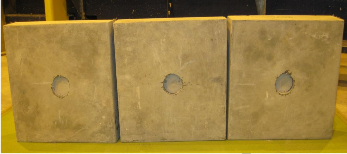
Figure 17: Typical failure on the loading side.
