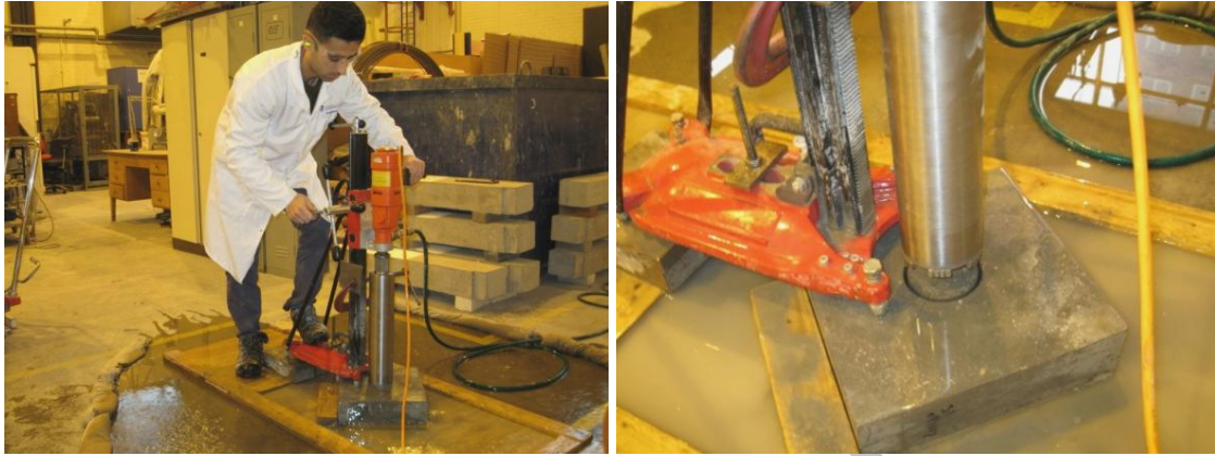
Figure 6: Specimen preparation, shear notch inducers using diamond drills
