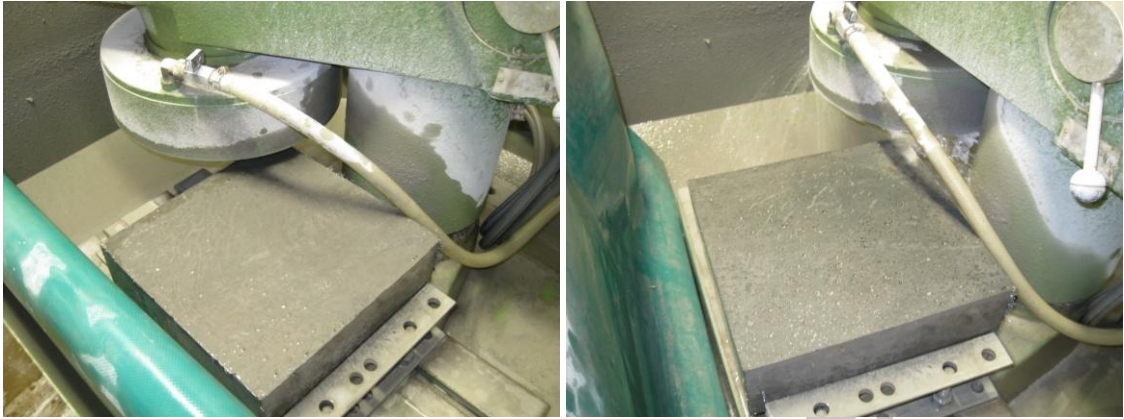
Figure 5: Specimen before and after grinding
