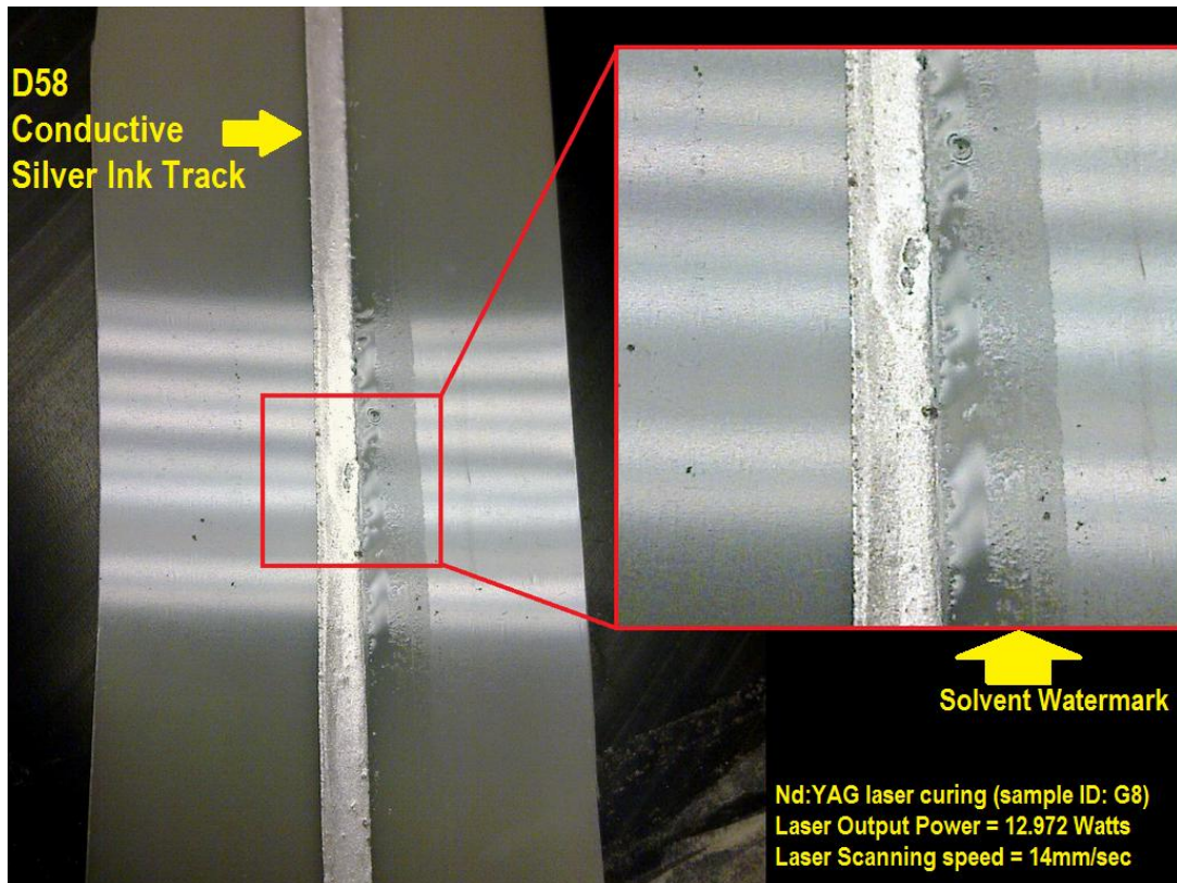
Figure 5.25: Solvent watermark observed at the edge of D58 silver ink track immediately after the laser cure process – the greater amount of expelled solvent liquid seen on one side is assumed to be as a result of the operation of the fume extractor system during the laser curing process.
