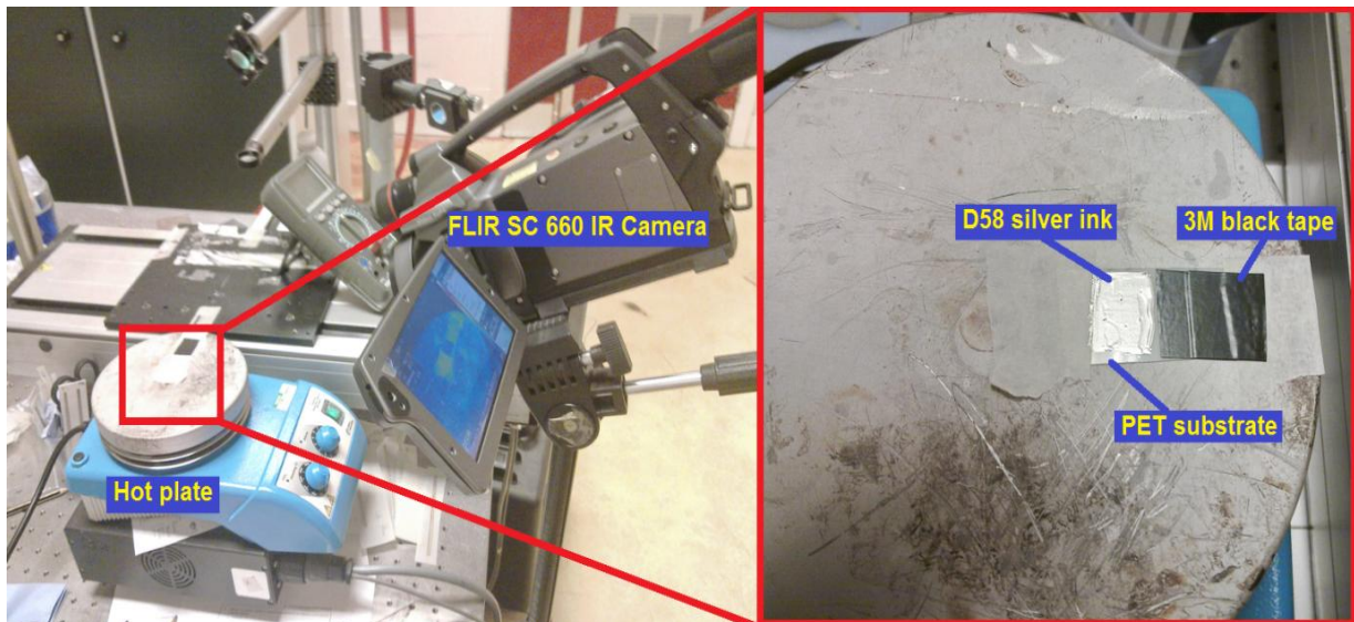
Figure 3.26: Experimental set-up for measuring emissivity of D58 silver ink.
