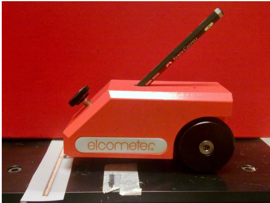
Figure 3.22: A conductive silver ink track was measured by Elcometer ® 501 pencil hardness tester for Wolff-Wilborn hardness test to measure ink track hardness property.
