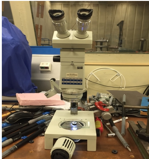
Figure 4-19 Microscope arrangement for observing the treeing propagation
