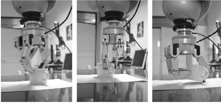
Figure 4.6. Resulting grasps (3 steps sequence): left - vision-based approach, middle - combined approach (first trial), right - combined approach (second trial). Adapted from Publication VI.
