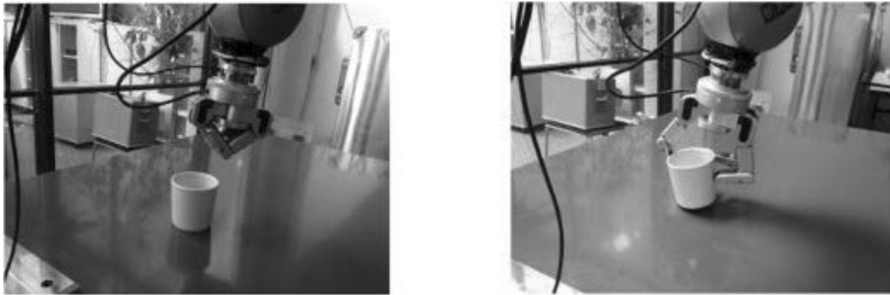
Figure 4.2. Resulting grasps: (left) Best single match; (right) Laplace model. Adapted from Publication V.
