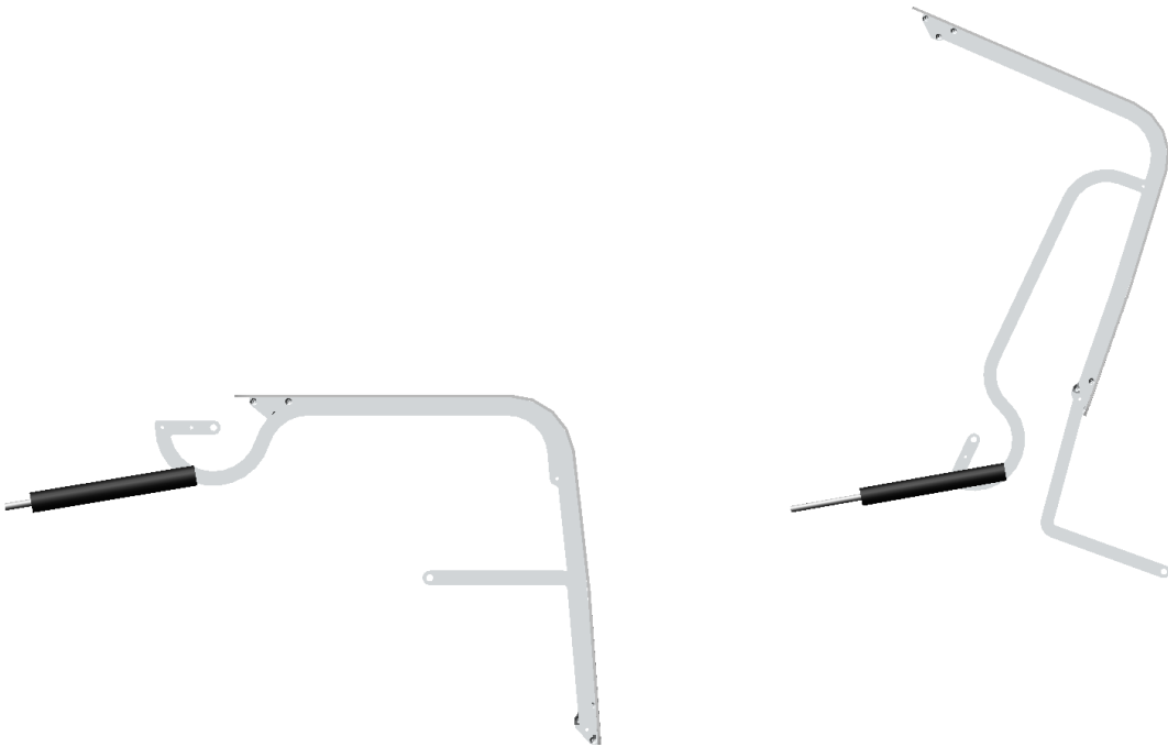
Figure 33: The ADAMS model with the gas spring, closed and open configurations
