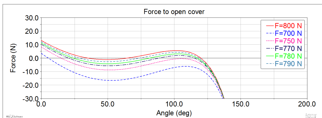
Figure 31: The force needed to open the main cover as a function of different spring forces between 700 N and 1000 N
