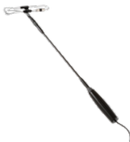
Figure 12: B&K 3595 sound intensity probe.
