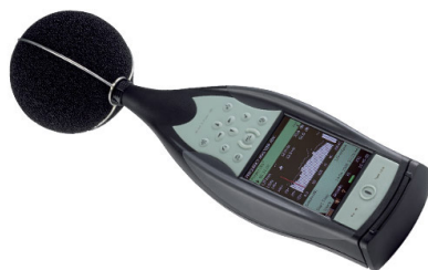
Figure 15: B&K 2250 sound level meter with microphone windscreen.
