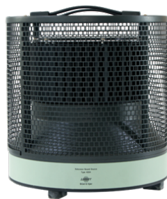
Figure 16: B&K 4204 reference sound source.
