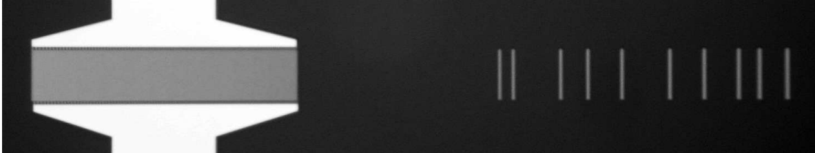
Figure 3.11: Photograph (taken through a microscope) of the fabricated UWB SAW tag device. The length of the structure is 1.1 mm.
