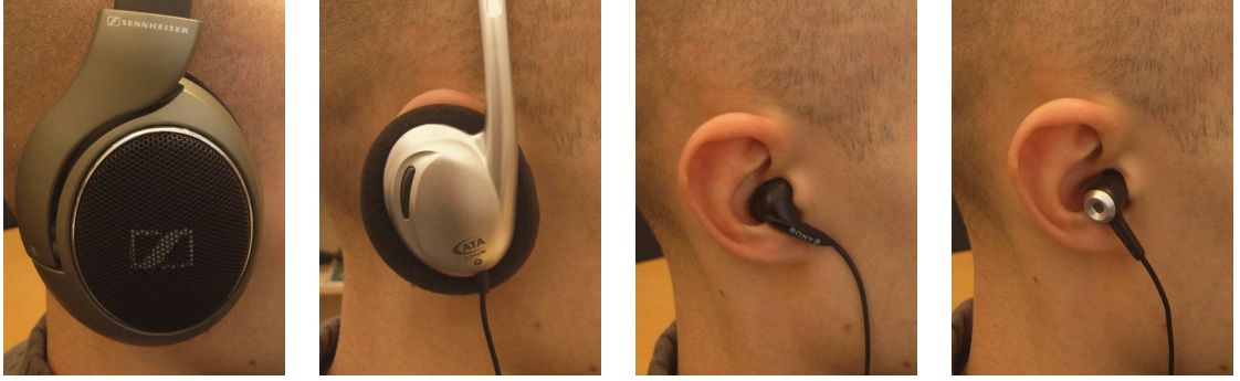
(a) Circum-aural head-phones. (b) Supra-aural head-phones. (c) Intra-concha head-phones. (d) Insert headphones.
