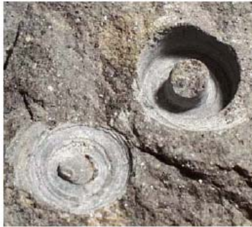
Figure 76: Mafurite drill holes. Note the unsuccessful drill-start of the left hole.
