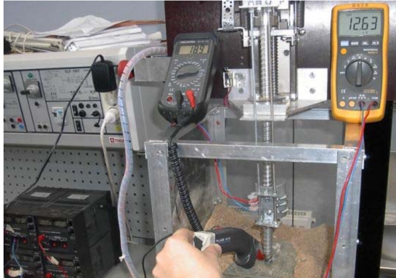
Figure 79: Temperature measurement setup (Image: MA).
