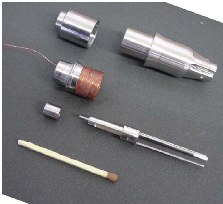
Figure 54: Old solenoid configuration [18]. The match (as a size-reference) is 42 mm long (Image: VTT).
