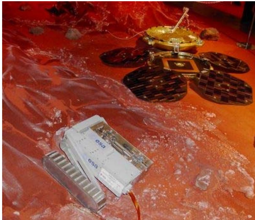
Figure 46: The MRoSA2 rover with Beagle-2 mock-up as a size-reference [24]. The length of the rover is 40 cm (Image: MA).
