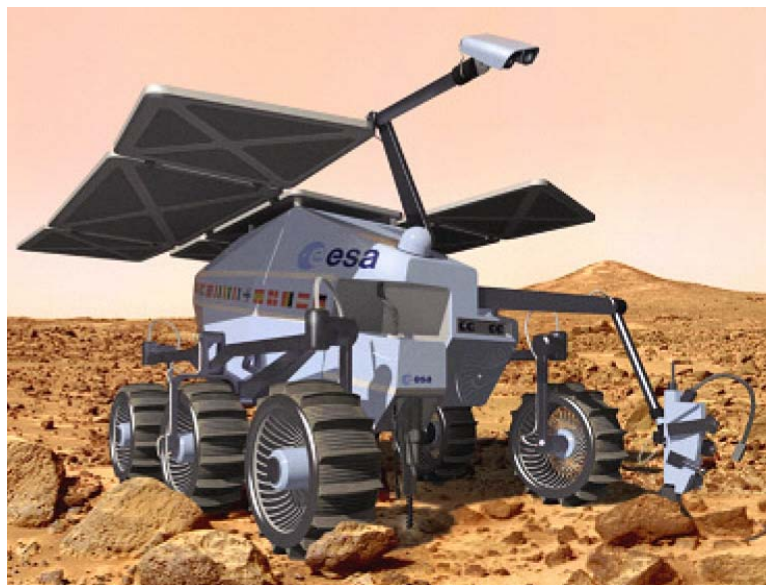
Figure 32: An artist's view of the ExoMars rover. The rover is approximately 1.5 m of height and weighs about 220 kg (Image: ESA).
