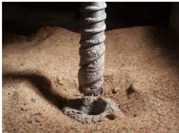
Figure 73: Drilling Diabase through a sand layer. The drill is 17 mm in diameter.
