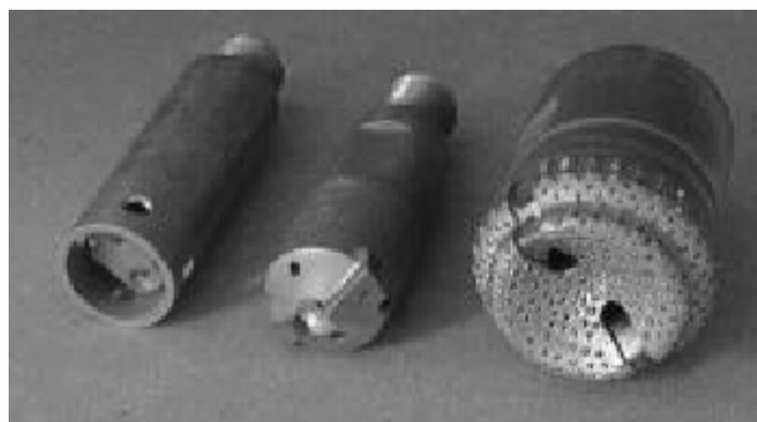
Figure 87: Terrestrial drilling bits: Drills (left to right): water jet, mechanically-assisted water jet and 50-mm diameter surface-set diamond bit (Image: Tempress Technologies Inc.).
