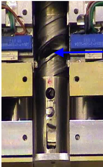
c) Raise tool from the tool carousel. Phase 5.
