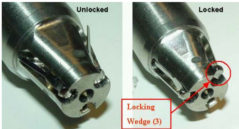
Figure 53: Solenoid driven mandrel hooks: Unlocked and locked position (Image: VTT).
