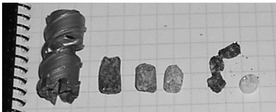
Figure 88: The MRoSA2 drill tool and five extracted core samples. Grid size of the paper behind the samples is 7 mm (Image: MA).
