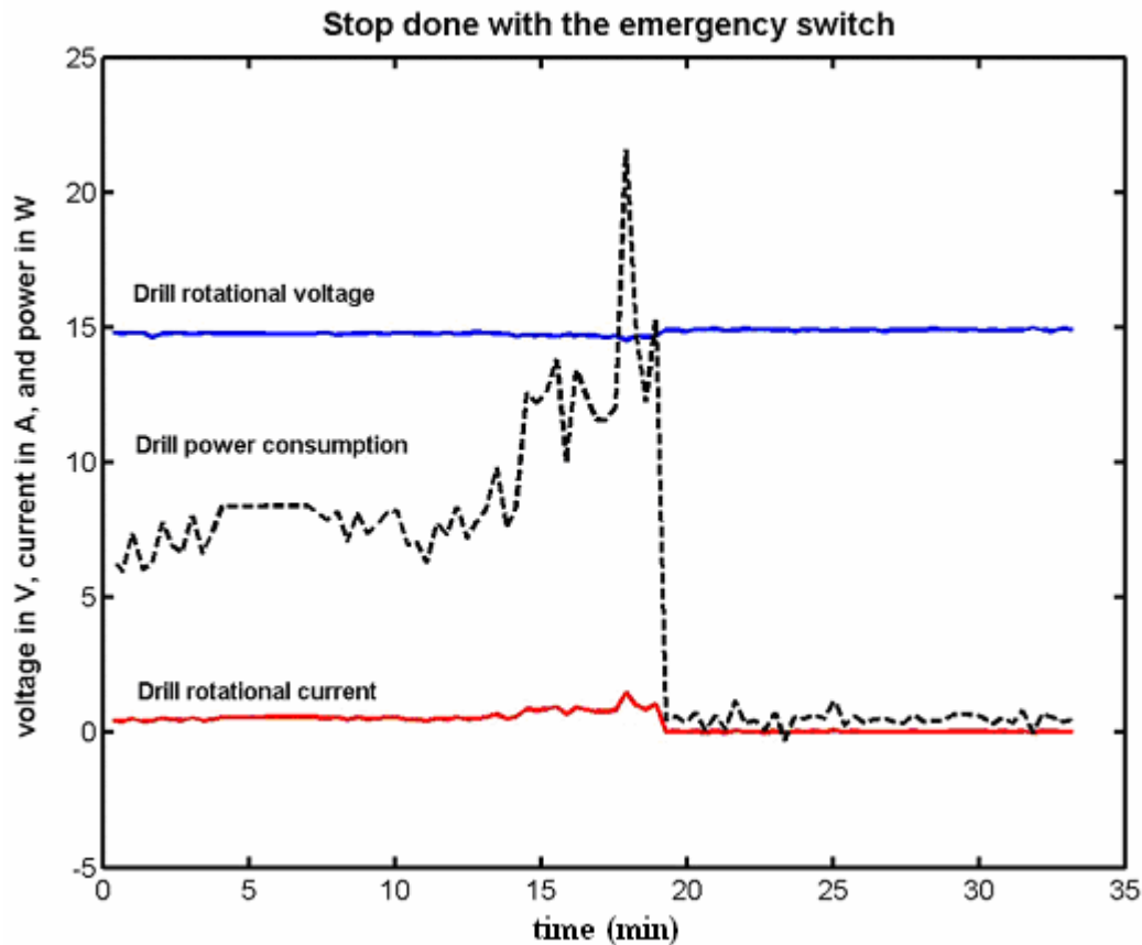
Figure 68: Emergency stop performed in a real situation when the drill started to wobble violently. The drill rotational voltage (blue), current (red), and power (black) are shown.
