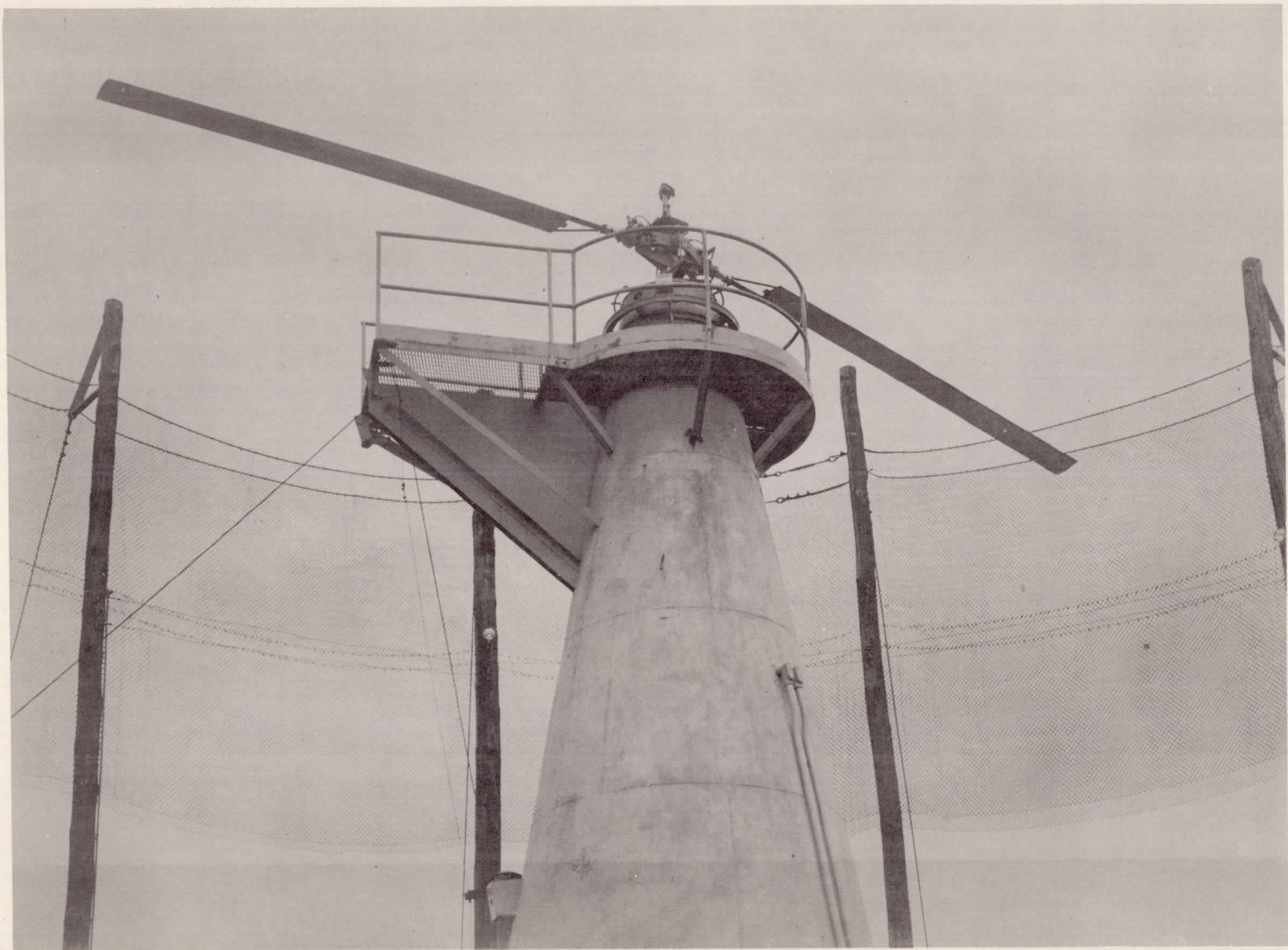
Figure 1.- Typical rotor blade installation on the Langley helicopter test tower.
