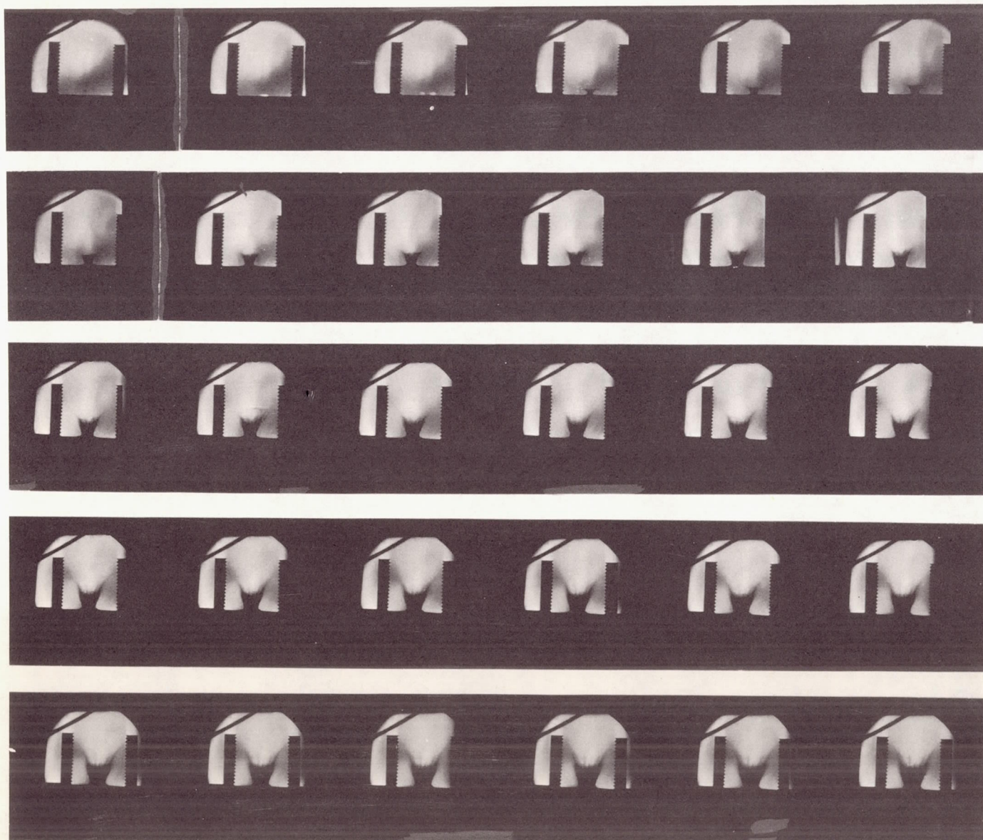
Figure 8.- High-speed framing camera records of an impact in basalt; framing rate = 1.04 \times 10^6 frames per second; impact velocity = 6.4 kilometers per second.
