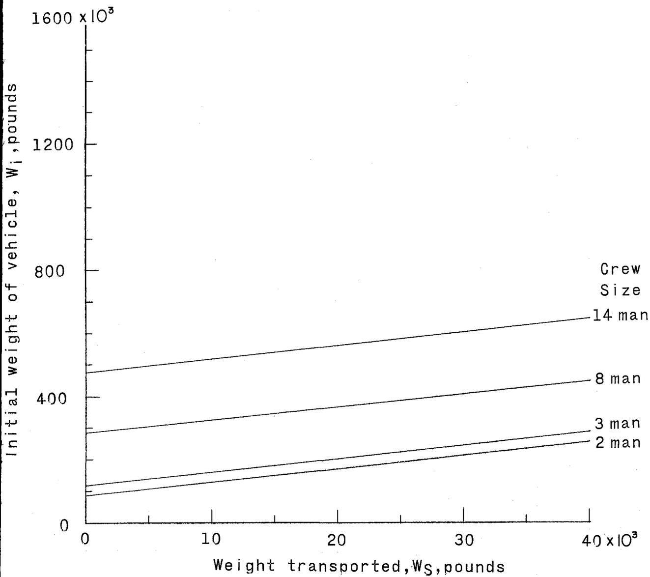
Figure 17.- Weight of direct lunar vehicle in transit to moon as a function of transported weight and crew size. 100-nautical-mile circular lunar orbit;  $I = 425$ .
