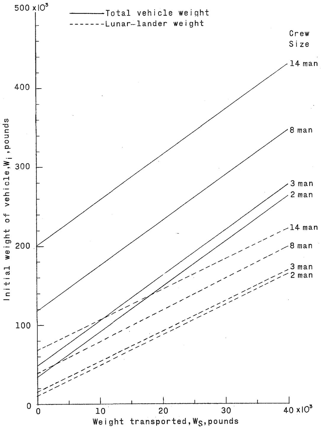
Figure 18.- Weight of lunar-orbit-rendevous vehicle and lunar lander in transit to moon as a function of transported weight and crew size. 100-nautical-mile circular lunar orbit;  $I = 425$  for entering and leaving lunar orbit;  $I = 315$  for landing and take-off from moon.
