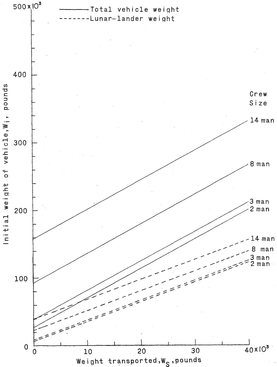
Figure 16.- Weight of lunar-orbit-rendezvous vehicle and lunar lander in transit to moon as a function of transported weight and crew size. 100-nautical-mile circular lunar orbit;  $I = 425$  for entering and leaving lunar orbit;  $I = 425$  for landing and take-off from moon.
