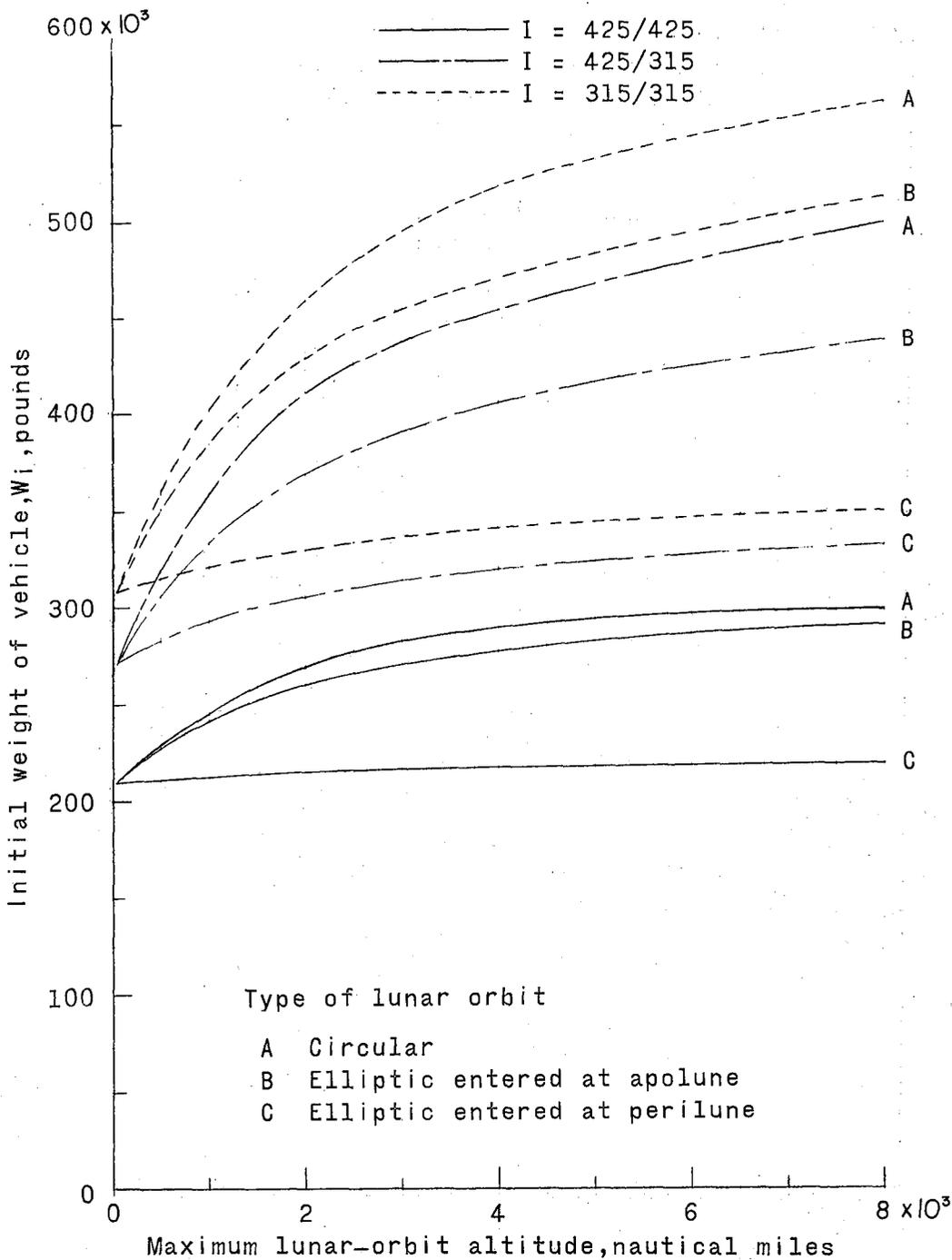
Figure 11.- Weight of lunar-orbit-rendezvous vehicle in transit to moon as a function of maximum lunar-orbit altitude for three types of lunar orbit and three combinations of fuel. Three-man crew; transported weight, 40,000 pounds.
