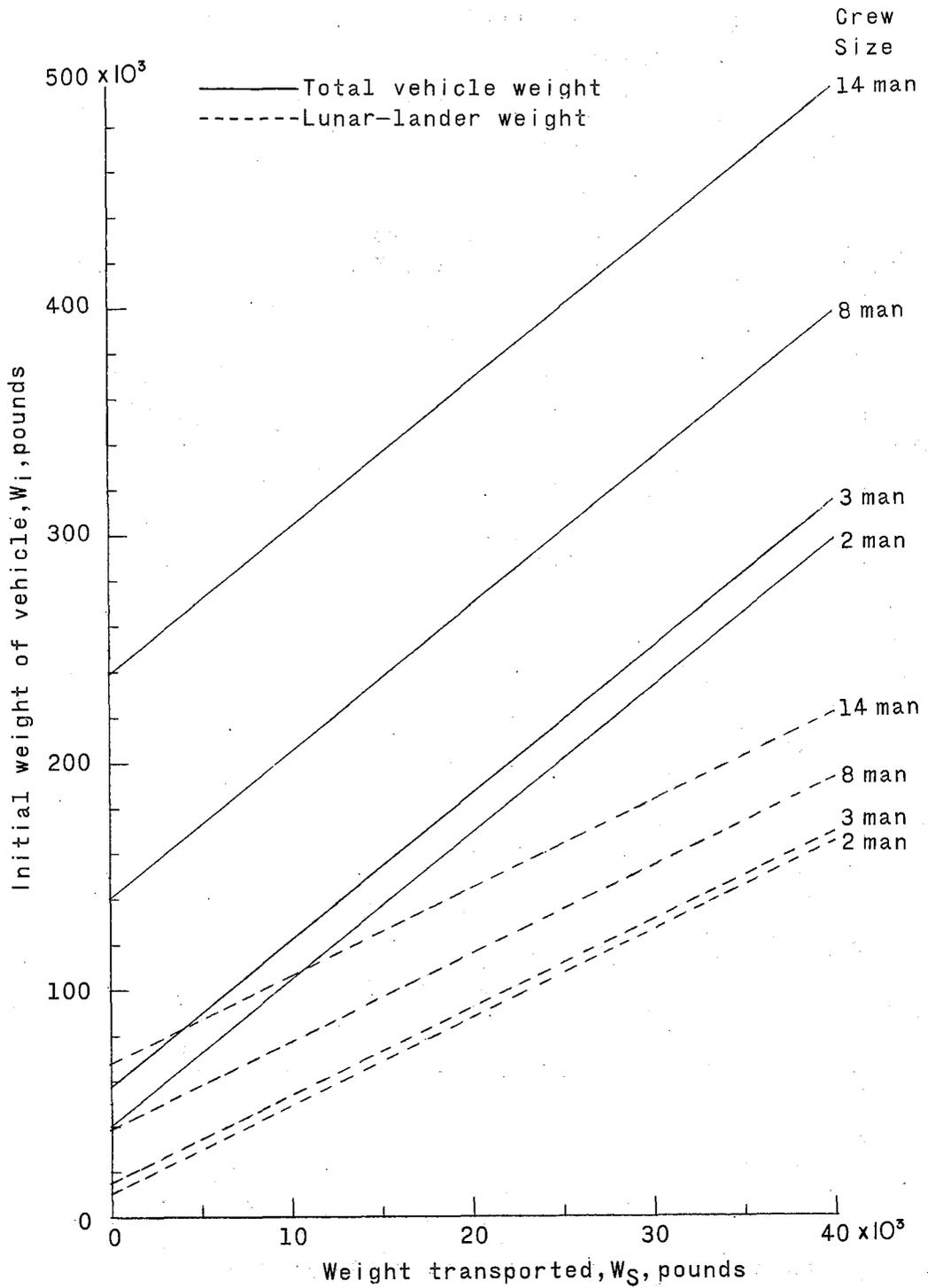
Figure 14.- Weight of lunar-orbit-rendezvous vehicle and lunar lander in transit to moon as a function of transported weight and crew size. 100-nautical-mile circular lunar orbit;  $I = 315$  for entering and leaving lunar orbit;  $I = 315$  for landing and take-off from moon.
