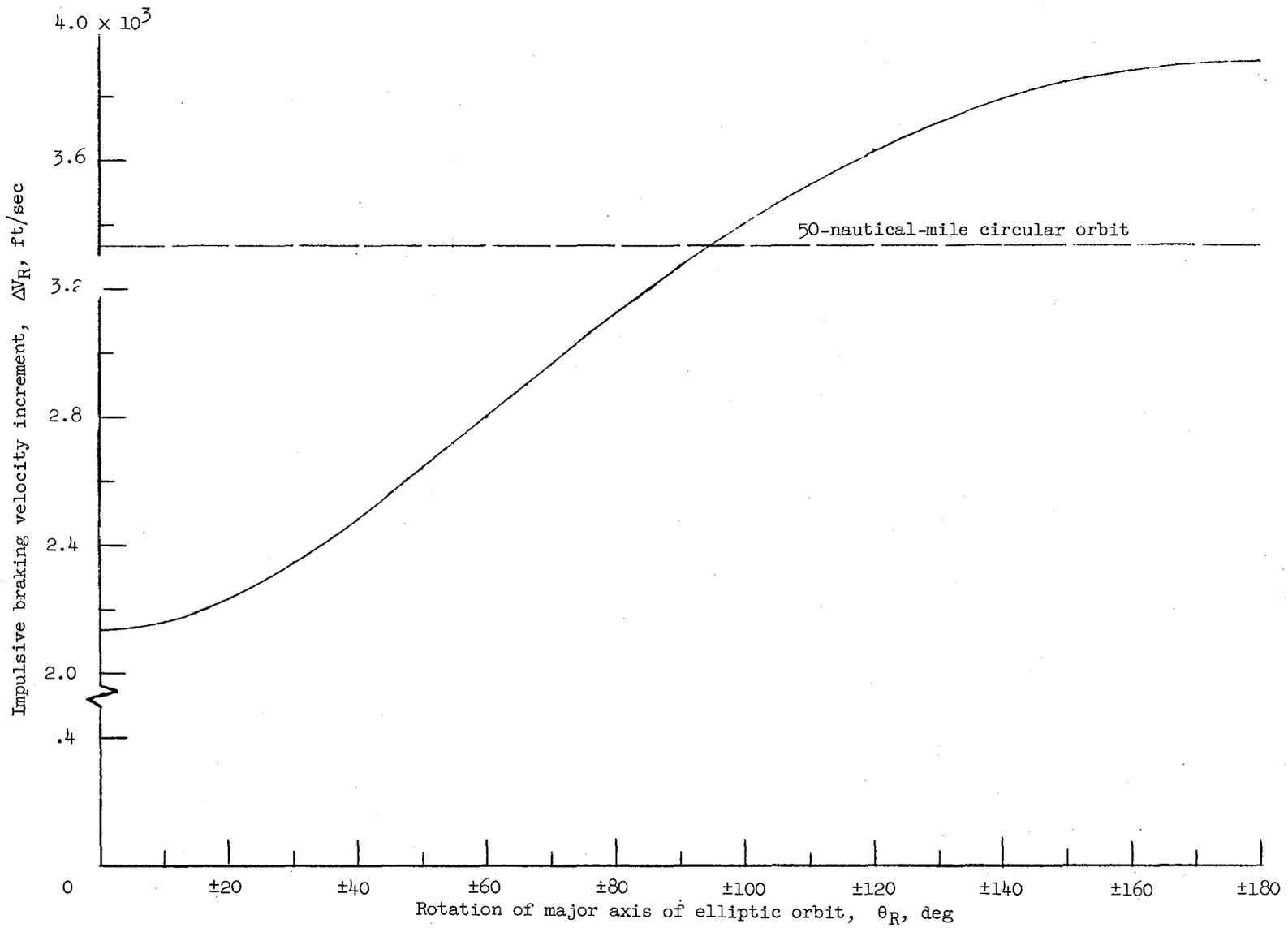
Figure 23.- Impulsive braking velocity increment as a function of rotation of the major axis of an elliptic orbit having a perilune altitude of 50 nautical miles and an apolune altitude of 2,000 nautical miles. Hyperbolic trajectory defined as having the energy level of 8,700 ft/sec at 50-nautical-mile altitude.
