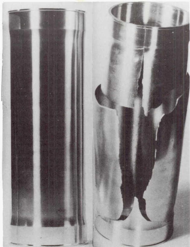
Fig. 8. Typical biaxial cylinder specimen: (left) before burst; (right) after burst.
