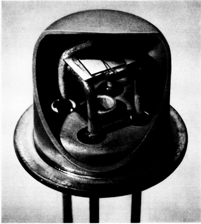
Fig. 6 — Construction of the radiation damage transistors.
