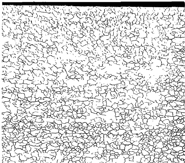
(a) 0.040-Inch-thick molybdenum specimen annealed at 2000° F in vacuum.
