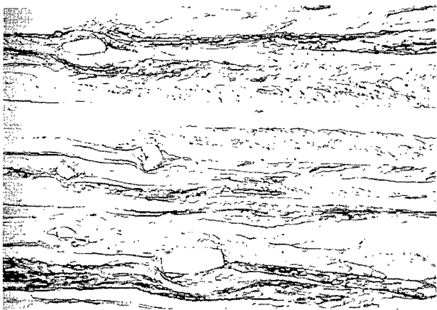
(c) Longitudinal section of 0.040-inch-thick molybdenum as received. X500.
