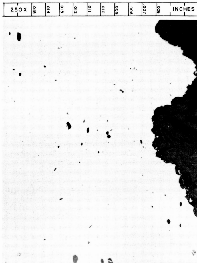
FIGURE 5 NECKED DOWN REGION OF TITANIUM 5% AL, 2.5% SN, EXTRA LOW INTERSTITIAL CONTENT, AFTER IRRADIATION TO 1 \times 10^{17} NVT AND FRACTURE AT 30° R, 250X
