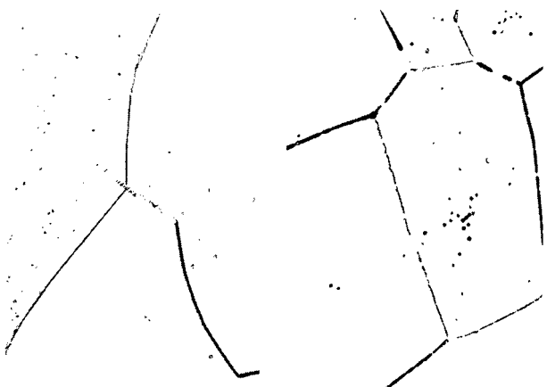
(c) Solution-treated and then aged 10 hours at 1800° F.
