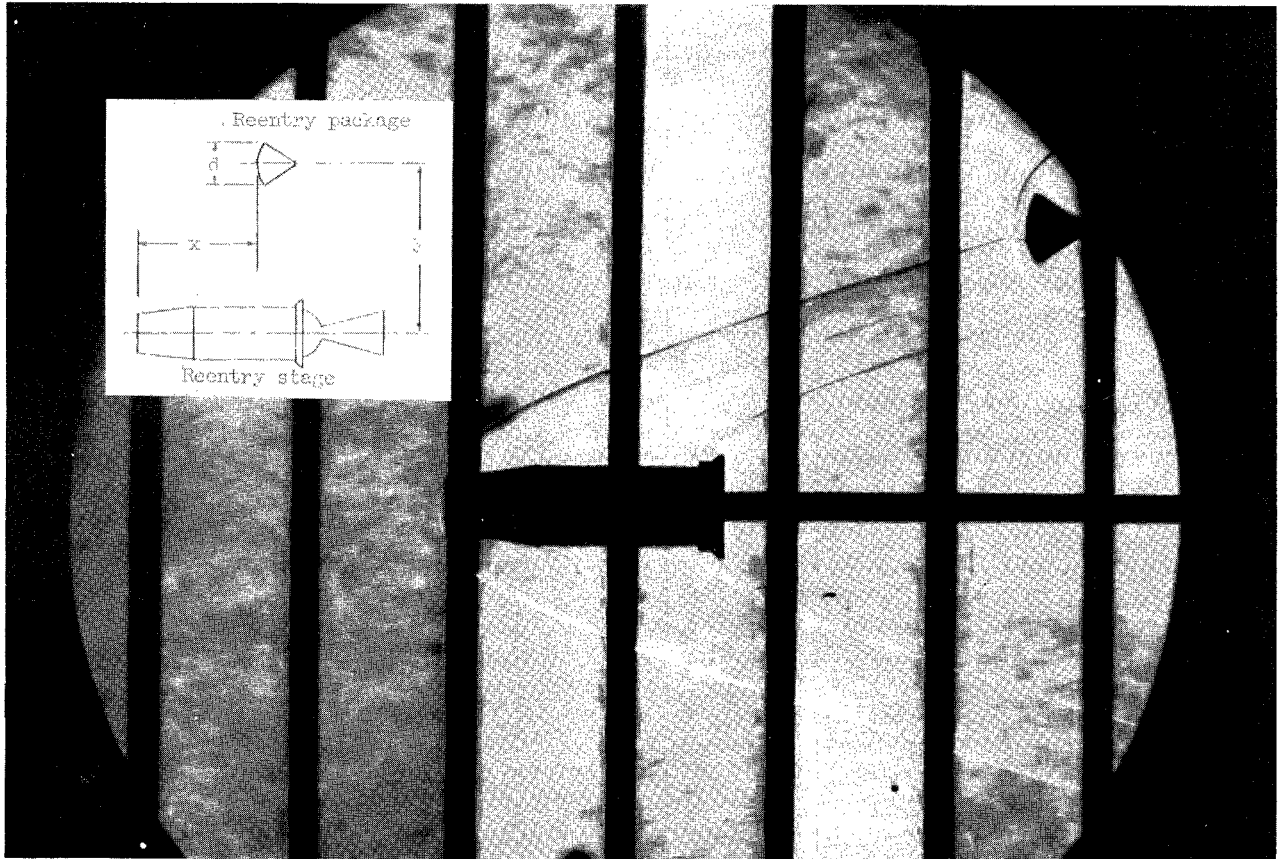
Figure 14.- Reentry-stage shock wave impinging on reentry-package at a Mach number of 4.60. y/d = 4 .
