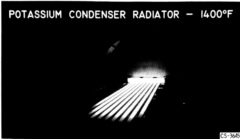
Figure 11. - Photograph of radiative condenser during operation at 1400° F vapor inlet temperature.
