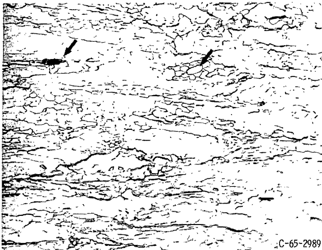
Figure 7. - Tungsten - 0.25 atomic percent boron annealed at 2700° F for 1 hour. Arrows point to recrystallized grains originating in vicinity of boride particles; X250. Reduced approximately 30 percent in printing.
