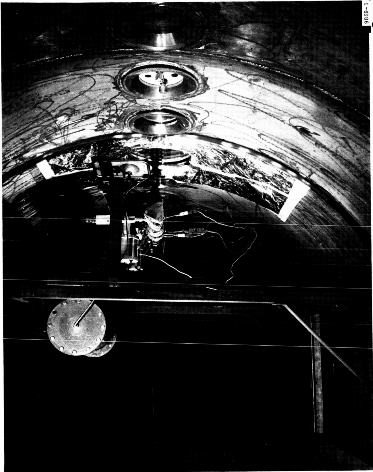
Figure 4-8. Flow System for N_2O_4 Tests (Inside Tunnel).
