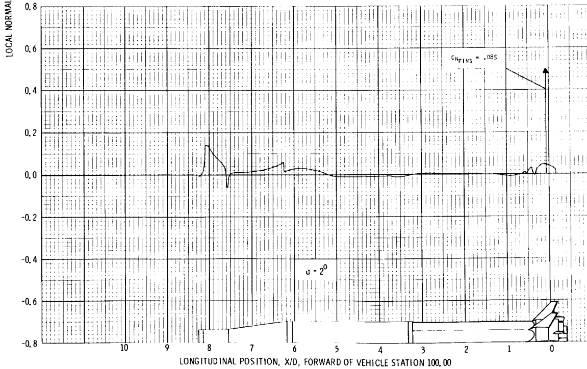
FIGURE 28: DISTRIBUTION OF LOCAL NORMAL FORCE COEFFICIENT AT MACH 1.57; \alpha = 2^\circ AND 4^\circ .
