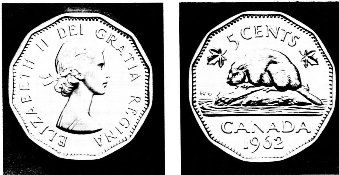
FIGURE 25. CANADIAN FIVE-CENT COIN MINTED FROM A BLANK PRODUCED BY SHERRITT GORDON FROM DIRECT-ROLLED NICKEL STRIP (REF. 170)
