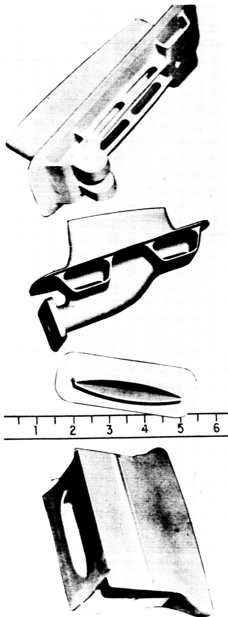
FIGURE 3. COMPLEX INVESTMENT CASTINGS OF A-286 PRODUCED BY MELTING AND CASTING UNDER VACUUM (REF. 37)
