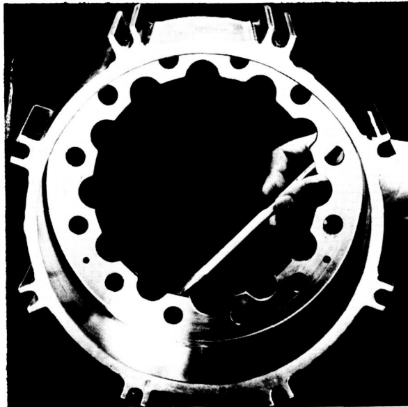
FIGURE 4. TORQUE TUBE CASTING OF CB-7Cu ALLOY FOR THE BOEING 707 BRAKE ASSEMBLY
