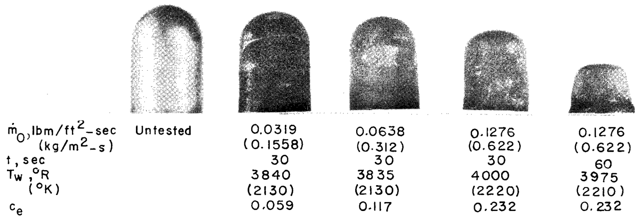
(b) 0.5-inch-diameter (1.27-cm) models exposed to high stagnation pressure of 6.4 atm.
