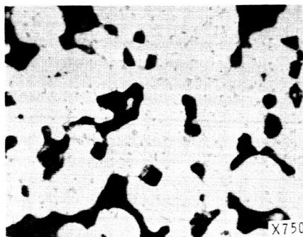
(C) DRY COMPACTED PREALLOYED POWDER COIN (1/8 IN. THICK). CLEANED WITH H 2 AT 800° F FOR 2 HR FOLLOWED BY 2 HR WITH H 2 AT 2300° F.
