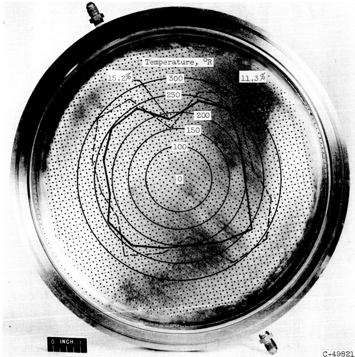
Figure 9. - Typical hydrogen temperature distribution at cooling-jacket outlet showing orientation with respect to injector (A) face plate. Chamber pressure, 150 lb/sq in. abs; mixture ratios, 11.3 and 15.2 percent hydrogen; inlet temperature, 51° R.
