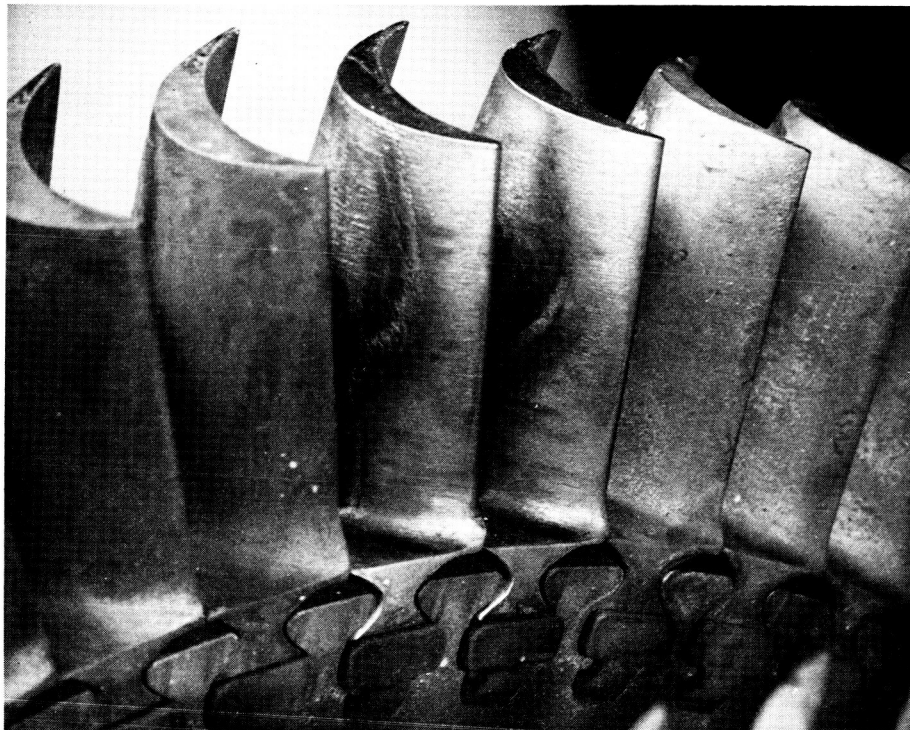
Figure 10. - Second-stage turbine rotor blades after 3000 and 5000 hours of operation with potassium vapor.
