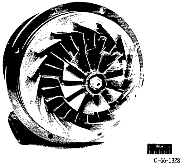
Figure 2. - Turbine stator and rotor assembly.
