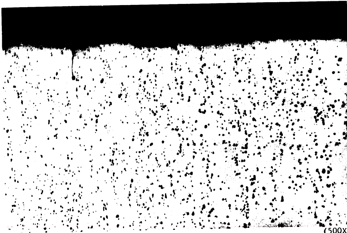
FIGURE 71. CROSS-SECTION OF EDM FINISH CUT AT 32,000 CPS. METAL REMOVAL RATE 0.045 CU. IN/HR.
