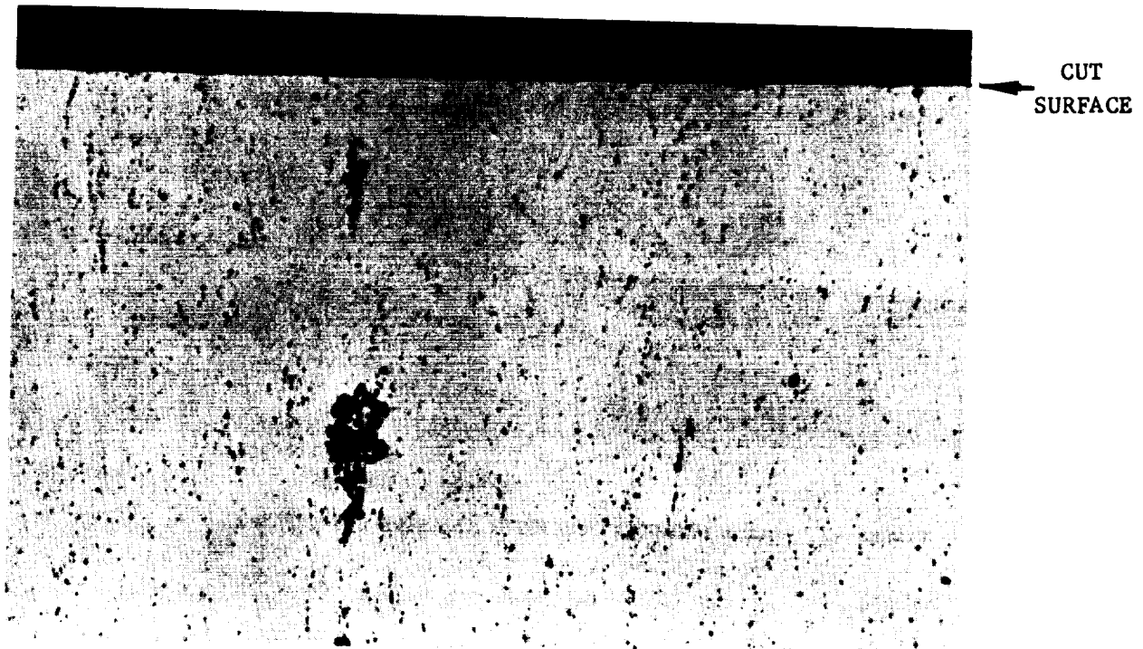
FIGURE 44. CROSS-SECTION OF SURFACE CUT DRY ON ABRASIVE WHEEL. FEED RATE 4.0 IPM AT 8,240 SFM. NOTE LARGE INCLUSION.
