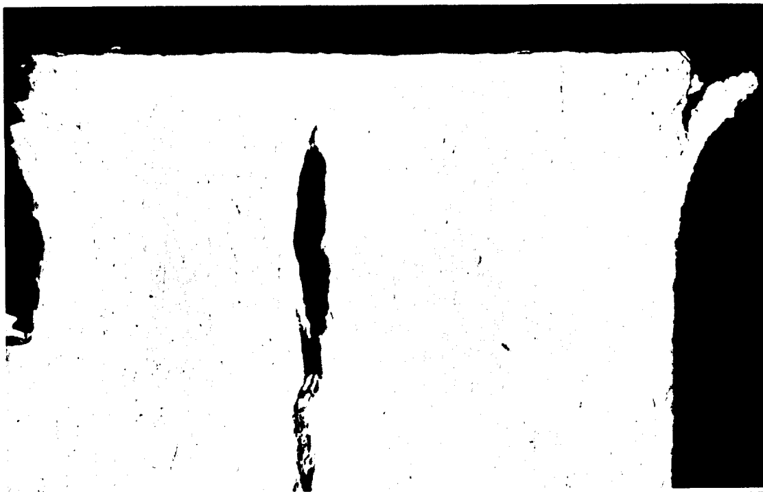
FIGURE 38. CROSS-SECTION THROUGH HOLE DRILLED WITH IMPROPERLY SHARPENED DRILL (UNETCHED)
