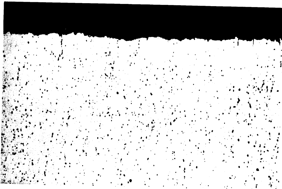
FIGURE 69. CROSS-SECTION OF EDM FINISH CUT AT 130,000 CPS. METAL REMOVAL RATE 0.125 CU. IN./HR.
