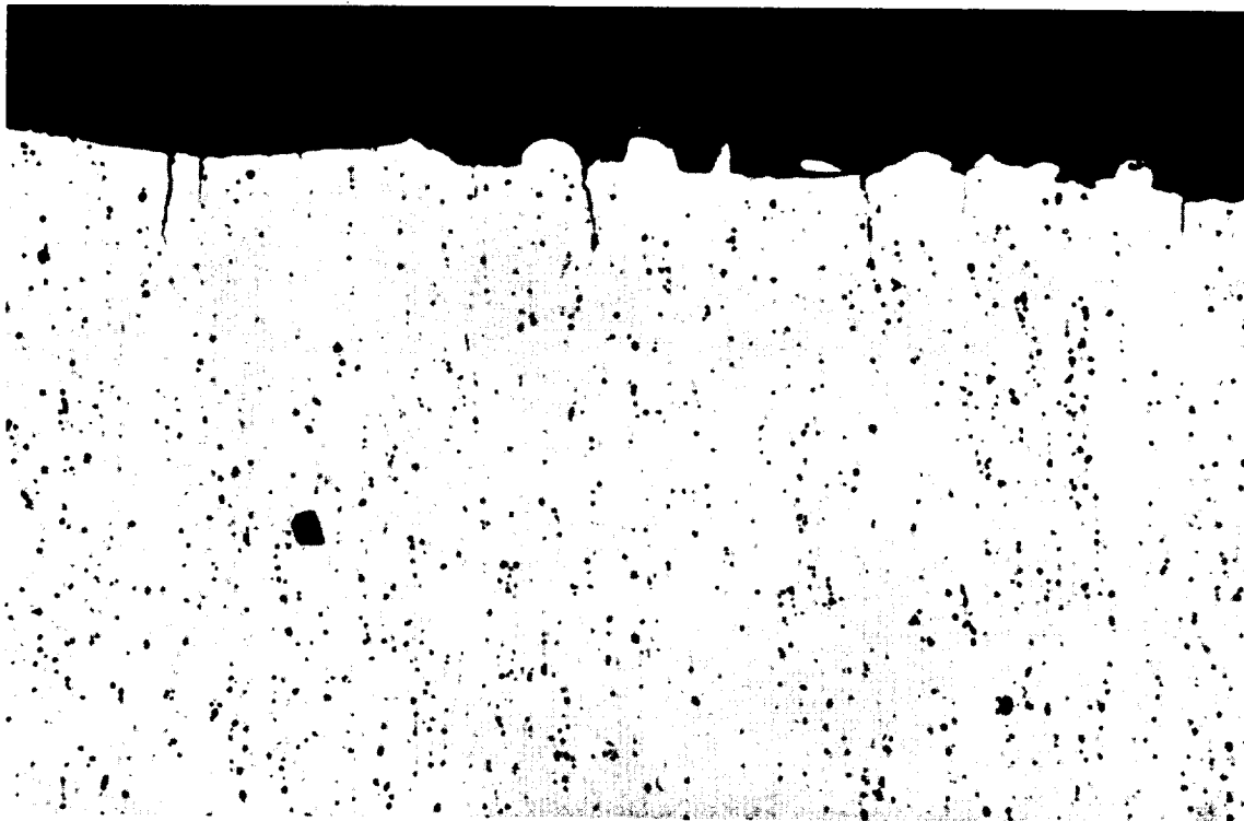
FIGURE 65. CROSS-SECTION OF EDM FINISH CUT AT 8,000 CPS. METAL REMOVAL RATE 0.38 CU. IN./HR.
