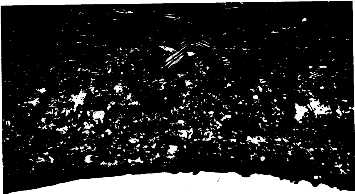
FIGURE 10. ENTRANCE SURFACE OF PUNCHED HOLE SHOWING EXTENSIVE DEFORMATION TWINNING (POLARIZED LIGHT)
