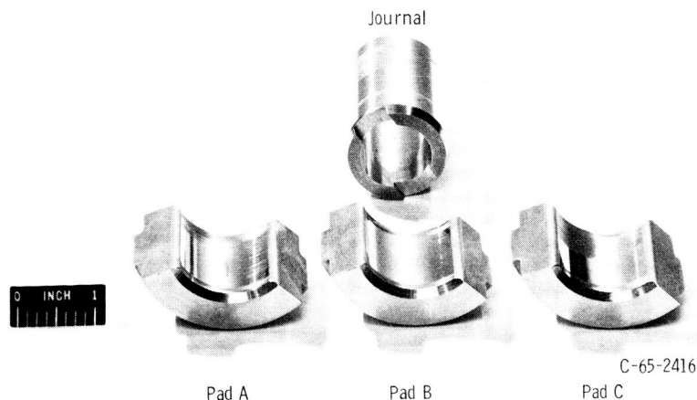
Figure 9. - Failure due to overloading. Tilting-pad bearing T-2 against journal J-12.
