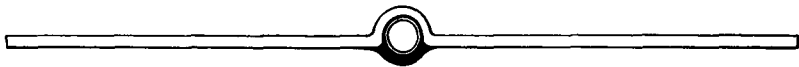
(g) Stamped full fin brazed to coated stainless-steel tube with part of tube covered with braze material.
