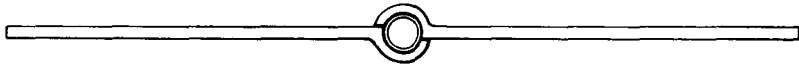
(e) Stamped half sections aluminum brazed to stainless-steel tube, precoated with titanium.
