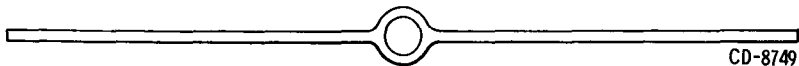
(h) All-aluminum finned-tube size machined from solid block used as reference for heat-rejection tests.
