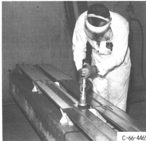
Figure 17. - Sandblasting a 40-foot finned-tube assembly prior to spray coating.
