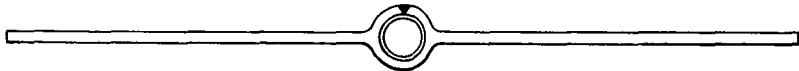
(d) Simulated extruded fin split and then tungsten-inert-gas welded after stainless-steel tube insertion.
