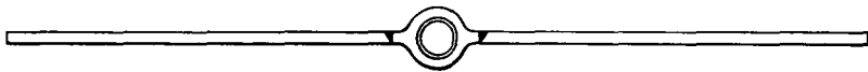
(f) Aluminum material cast around stainless-steel tube with fin welded to aluminum casting.
