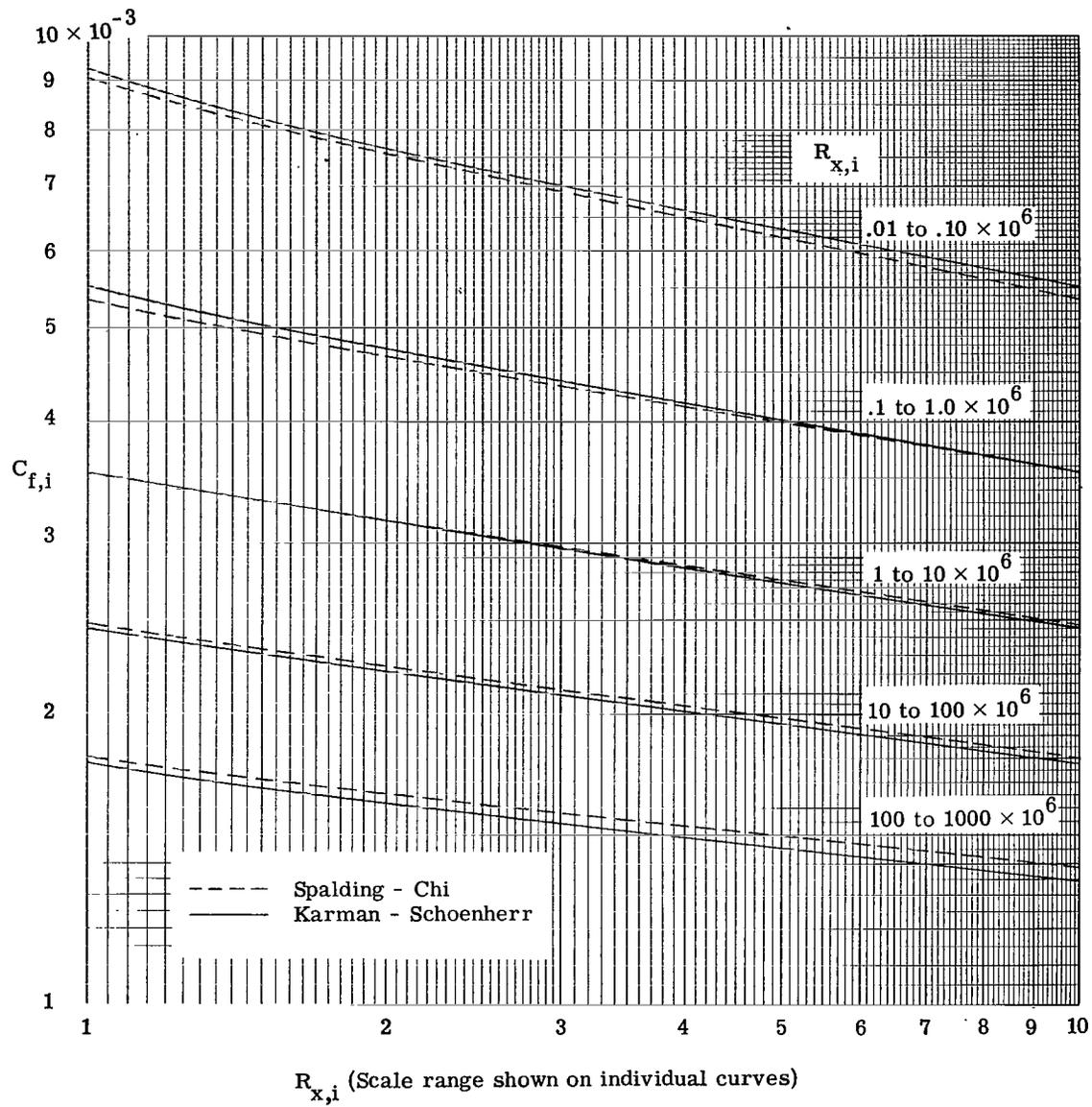
Figure 3.- Variation of incompressible local skin-friction coefficient with Reynolds number.
