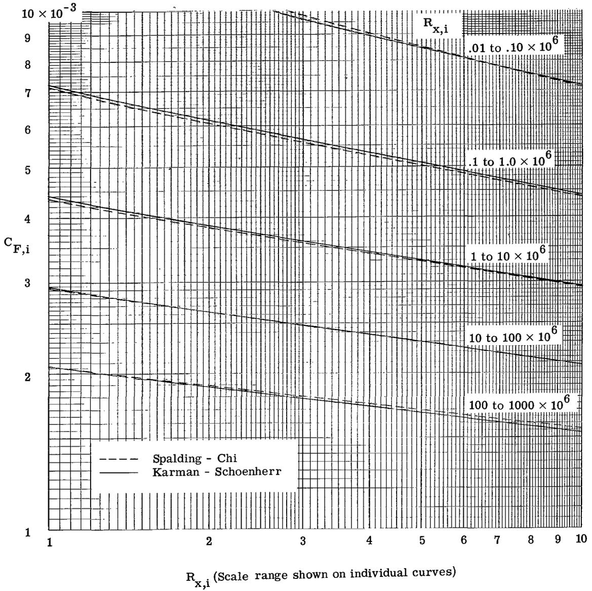
Figure 4.- Variation of incompressible average skin-friction coefficient with Reynolds numbers.
