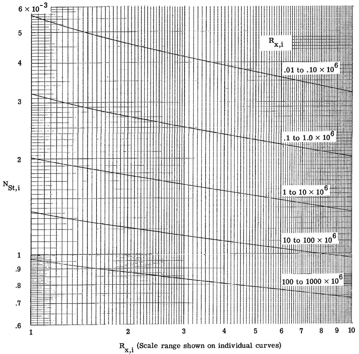
Figure 2.- Variation of incompressible Stanton number with Reynolds number based on the Karman form of the Reynolds analogy equation and the Karman-Schoenherr skin-friction equation.  $N_{Pr} = 0.725$ .
