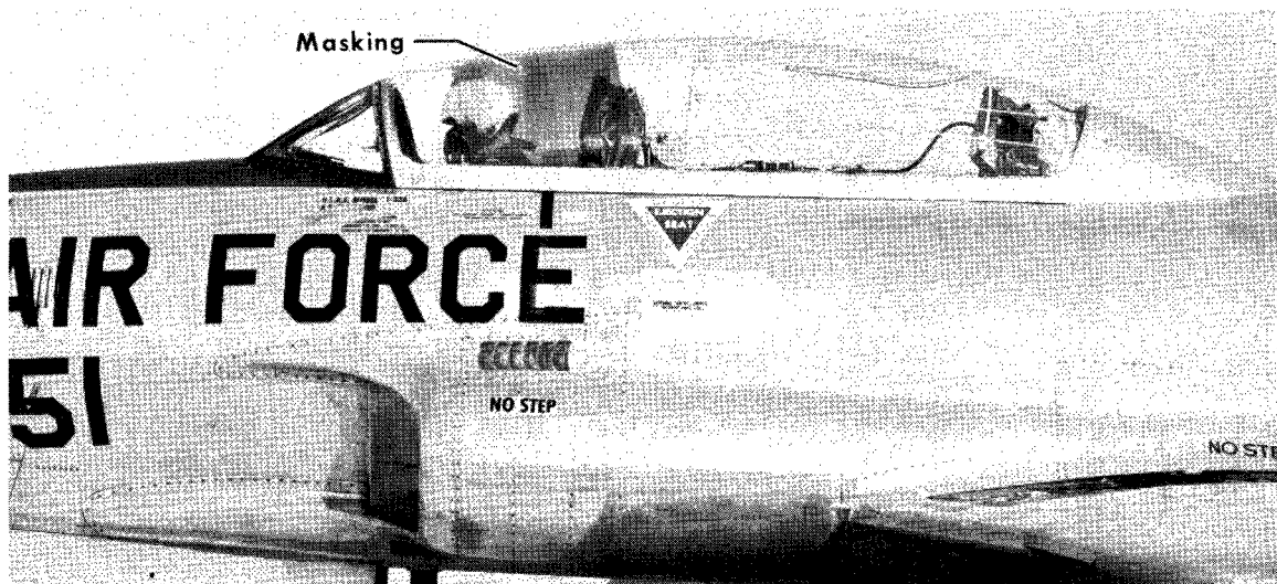
(a) Closeup side view of T-33A showing cockpit masking and subject pilot.
