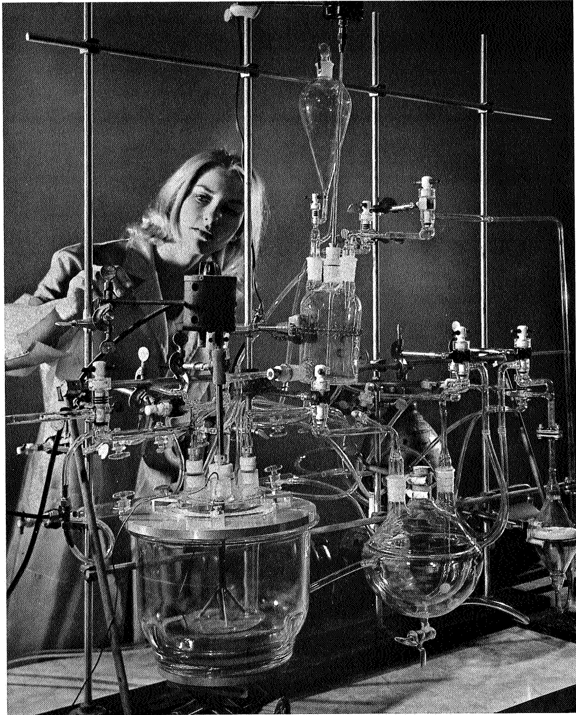
Figure 13. Laboratory Magnesium Mirror Electroforming Assembly
