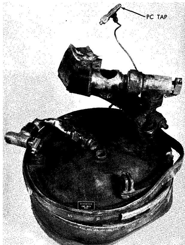
Figure 36—Flight 4.113 GA-GI aft fuel tank bulkhead showing burned aniline deposits.
