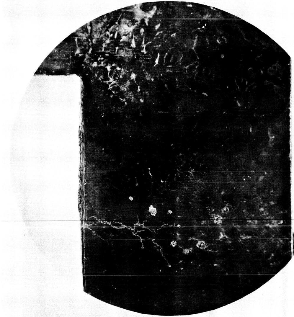
Figure 8(b). - 15X magnification of same area of figure 8(a) showing cracked area and high point material.
