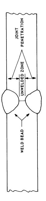
FIGURE 1. CROSS SECTION OF BUTT JOINT SHOWING INCOMPLETE PENETRATION
