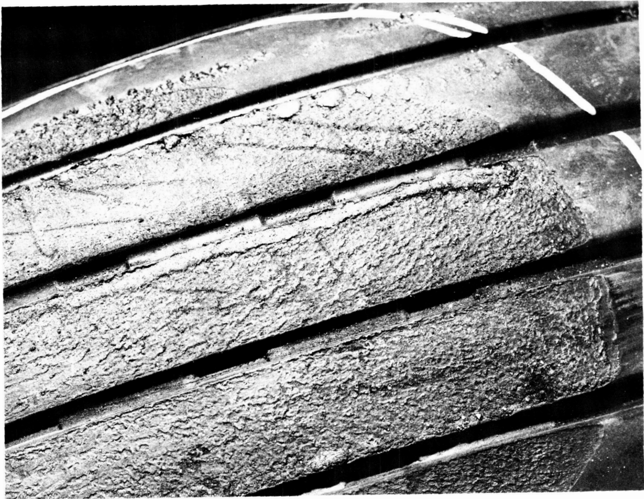
Figure 20.- Reverted-rubber skid patch obtained with four-engine jet transport on wet runway.
