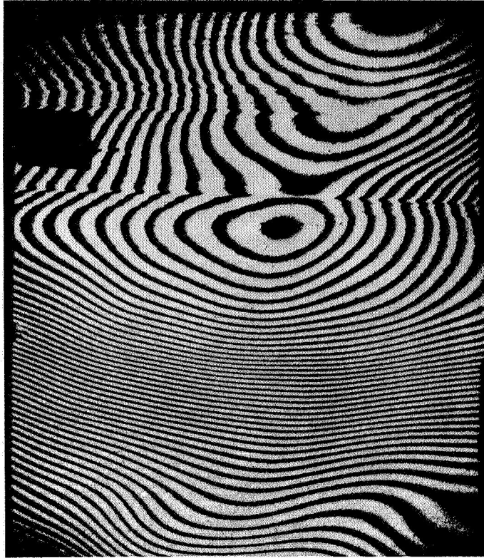
Figure 32. Interferential Holography in Diffuse Light. The hologram recorded according to Figures 30 and 31 reconstitutes an interferogram of the phase object O which has been recorded. In this case the object is a glass plate whose 'grains' and whose variations of refractive index and thickness are visible. The hologram obtained in this manner shows all the properties of the ordinary holograms in diffuse light, in particular, the interferogram is directly visible to the naked eye.
