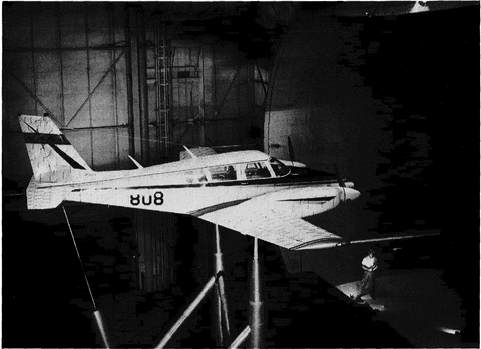
Figure 3.- Photograph of airplane mounted in Langley full-scale tunnel.
